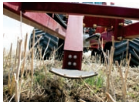
A paddle sensor rides above the ground to detect stubble rows.
