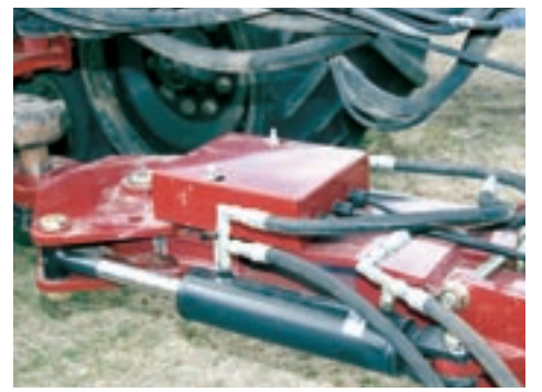
Hydraulic cylinders move the frame to keep the openers between the rows
