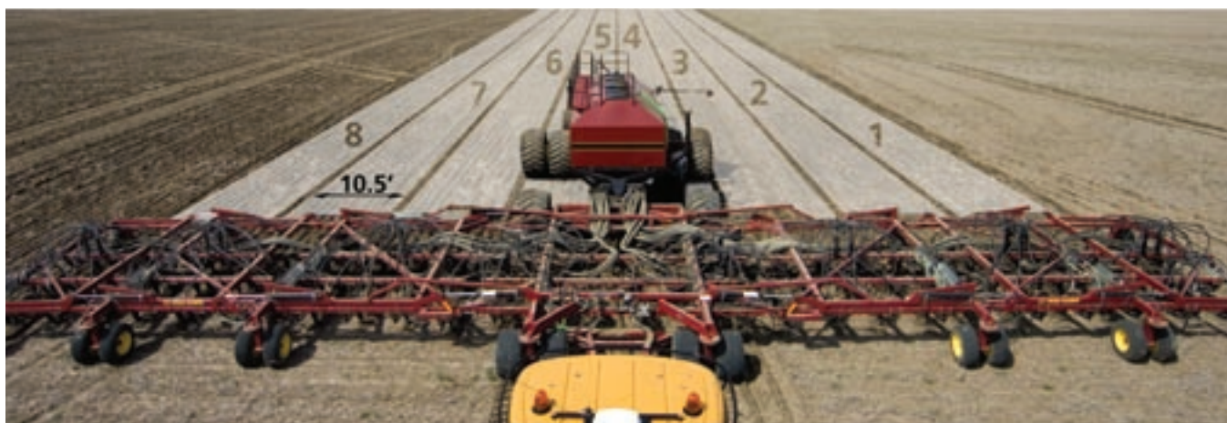
With SCT the section size that is turned on and off is determined by the width of the toolbar. For example, an 84-foot wide drill (shown above) each section would be 10.5 feet wide.
