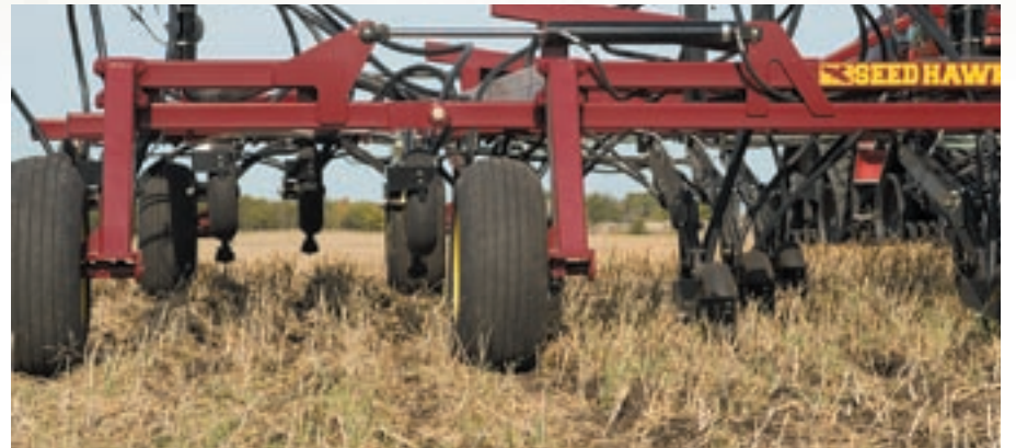
Openers lift and meter gate sections close when a section of the drill overlaps seeded ground.
